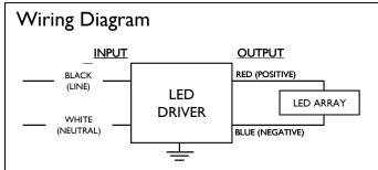
Input and output use lead-wires. Lead-wires are 18AWG 105C/600V solid copper
